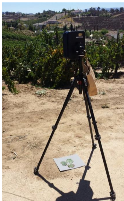
Figure 1. Portable hyperspectral imaging system (SOC710-VP ® ) and imaging off-the-vine leaves in the field.
