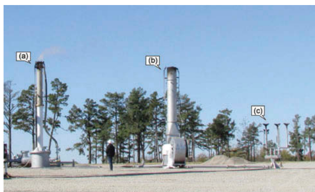
Figure 1. Three flares used in the experiment: (a) QFS steam-assisted flare; (b) AFDS air-assisted flare; and (c) MPGF multi-point sonic flare.
