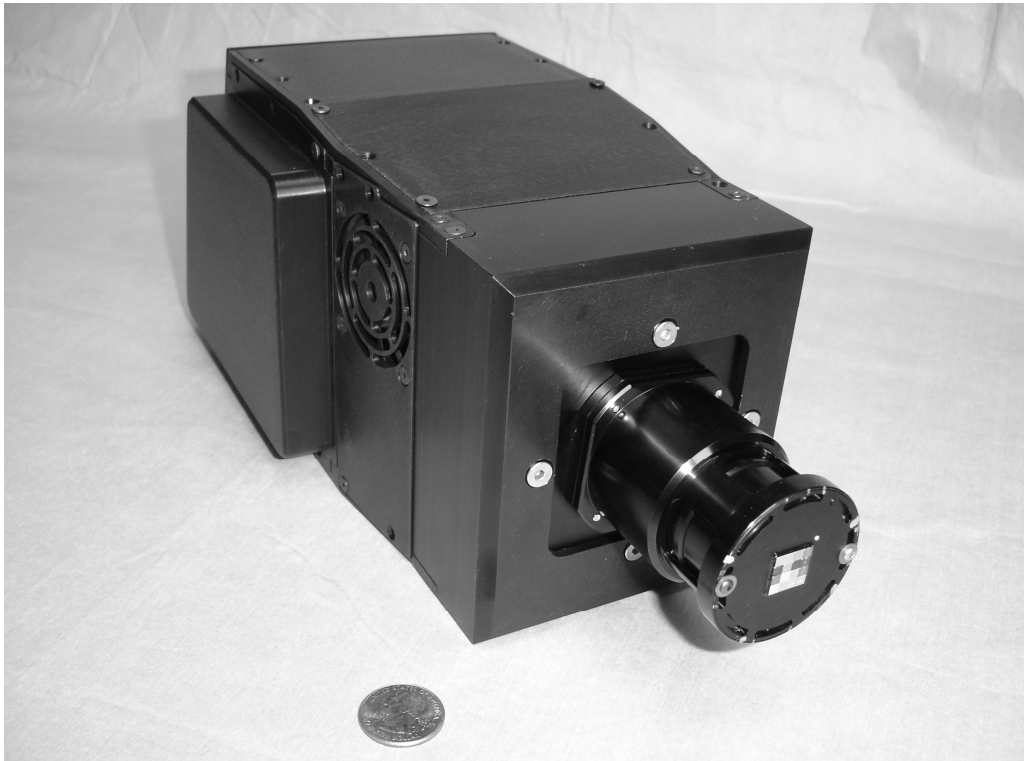
Figure 8: The Hypersensor camera installed with the hyperspectral video processor system is a compact data collection system that requires only a display, keyboard and mouse to operate.
