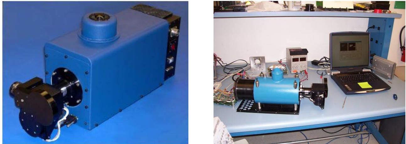
Figure 1: MWIR HSI fully assembled (left) and under test in the lab (right)
