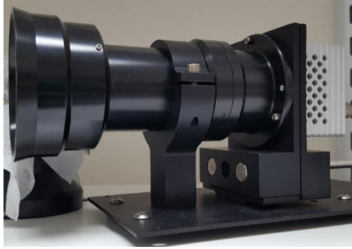
Figure 3a. SOC's VNIR Hypersensor Imager – Data cube is 512 x 512 spatial pixels x 16 filters. Filters can be any combination of spectral and polarimetric. Sensor operates from 400nm – 950nm.
