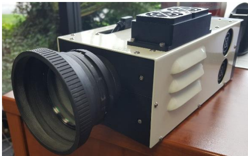
Figure 3b. SOC's SWIR Hypersensor Imager – Data cube is 320 x 256 spatial pixels x 16 filters. Filters can be any combination of spectral and polarimetric. Sensor operates from 0.9 \mu m – 1.7 \mu m.
