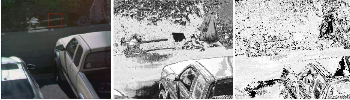
Figure 1. SWIR Image of Truck – Reference image in RGB (left), SWIR DoLP (center) and SWIR AoLP (right).
