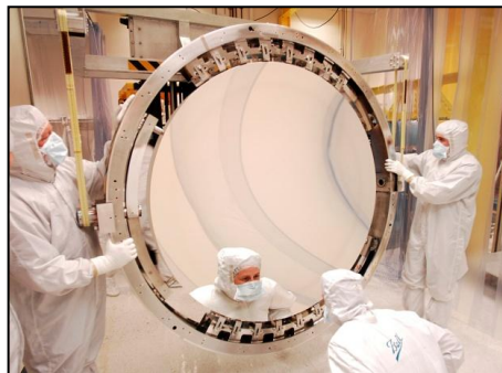
1.5m Kepler Primary, Coated w. Protected Ag, for Ball/NASA
