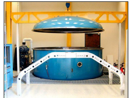
SOC Chamber for Parts up to 3 meters
