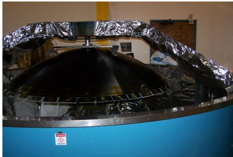
Reflector installed in chamber, ready for coating
